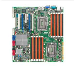
**Asus KGPE-D16 Dual Socket G34/ AMD SR5690/ V&2GbE/ SSI EEB Server Motherboard KGPED16ASMB4IKVM**
