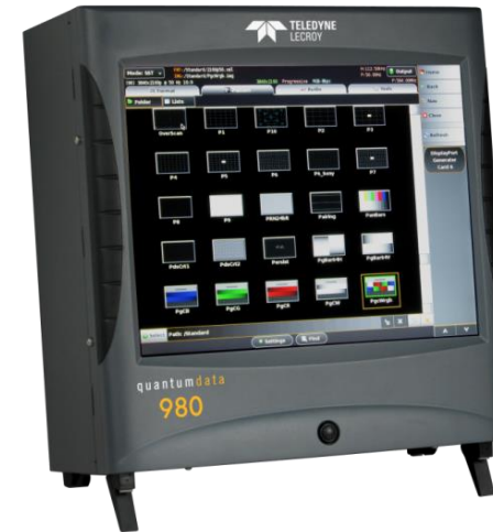
980B Platform w/ DisplayPort 1.4 Protocol Analyzer module
