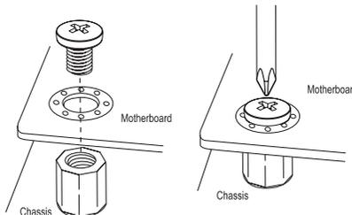
6. Using the Phillips screwdriver, insert a Pan head #6 screw into a mounting hole on the motherboard and its matching mounting hole on the chassis.
