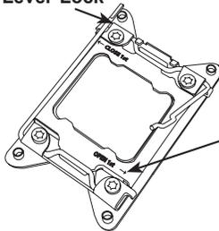
Push down and lock the lever labeled "Open 1st"
