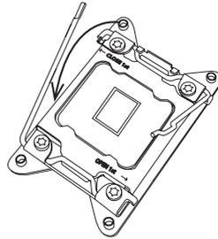
3. With the lever labeled "Close 1st" fully retracted, gently push down on the lever labeled "Open 1st" to open the load plate. Lift the load plate to open it completely.
