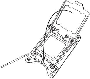
**2** Push down and lock the lever labeled "Close 1st"
