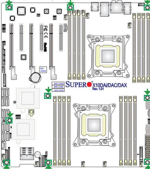
**Warning:** 1) To avoid damaging the motherboard and its components, please do not use a force greater than 8 lb/inch on each mounting screw during motherboard installation. 2) Some components are very close to the mounting holes. Please take precautionary measures to prevent damage to these components when installing the motherboard to the chassis.
