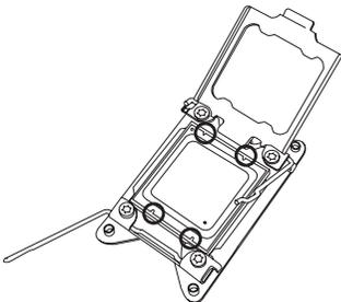
**Warning:** You can only install the CPU inside the socket in one direction. Make sure that it is properly inserted into the CPU socket before closing the load plate. If it doesn't close properly, do not force it as this may damage your CPU. Instead, open the load plate again to make sure that the CPU is aligned properly.
