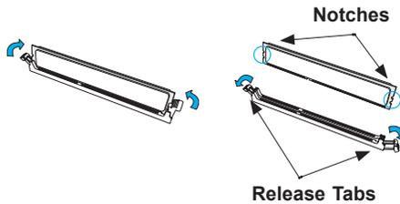
3. Align the key of the DIMM module with the receptive point on the memory slot.
