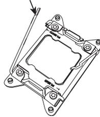
8. Close the load plate with the CPU inside the socket. Lock the lever labeled "Close 1st" first, then lock the lever labeled "Open 1st" second. Using your thumb, gently push the load levers down to the lever locks.
