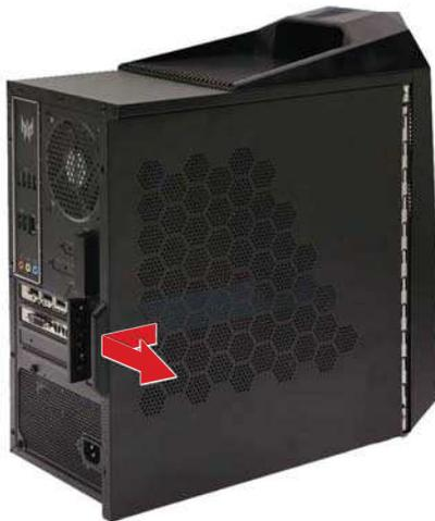
4. Detach the side panel from the unit and put it aside for re-installation later.
