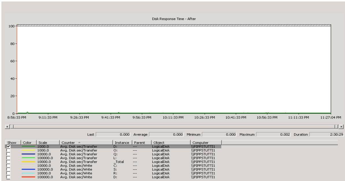
This dramatic reduction in response time leads to a dramatic reduction in queue depth, not because the application can send more parallel requests but because its response from storage is so fast that it can't develop a very deep queue, as seen in the queue depth "after" screenshot.
