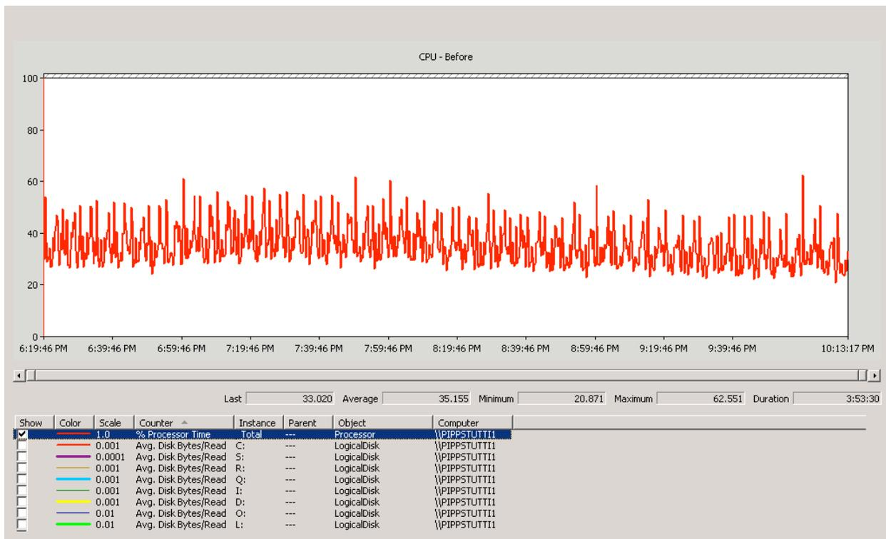
After the insertion of SSDs, there was a dramatic increase in CPU utilization to 46%, close to a 50% improvement in CPU utilization. With SSD you will find that I/O performance should scale linearly with CPU load.
