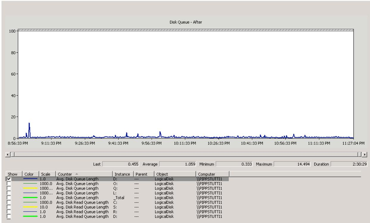
These screenshots indicate that the customer saw a dramatic performance improvement from implementing SSD. They show that instead of scaling out by adding more drives and servers, users can scale up by adding SSD. As mentioned previously, scaling up is usually simpler and more cost effective than scaling out.
