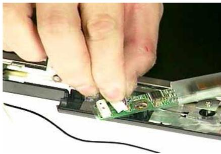
Disassembling LCD panel
