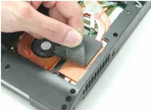
2. Remove 4 screws aside the CPU. And take away the thermal module.
