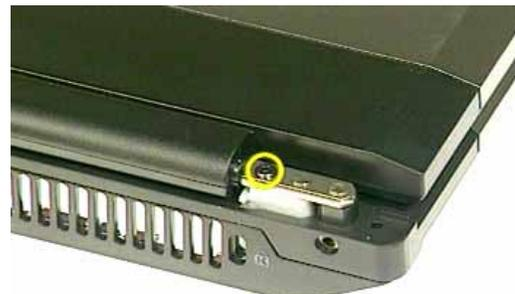
7. Remove the LCD module from system.
