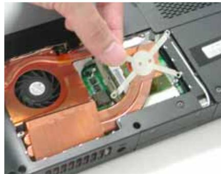
3. Remove the CPU slot and take away the CPU.
