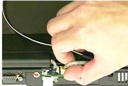
5. Remove 1 screw and disconnect the connector.
