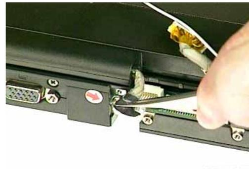
6. Remove 2 screws on both ends.
