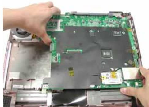
Removing Modem board
